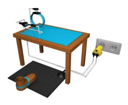
Static dissipative matting is specially formulated to drain static electricity from workers, thereby avoiding unpleasant static shock while safeguarding equipment. To achieve an ESD protective work area, all conductors, including personnel, must be grounded.
