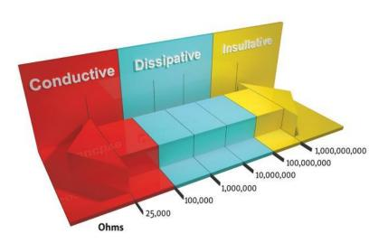
Static dissipative matting is specially formulated to drain static electricity from workers, thereby avoiding unpleasant static shock while safeguarding equipment.
